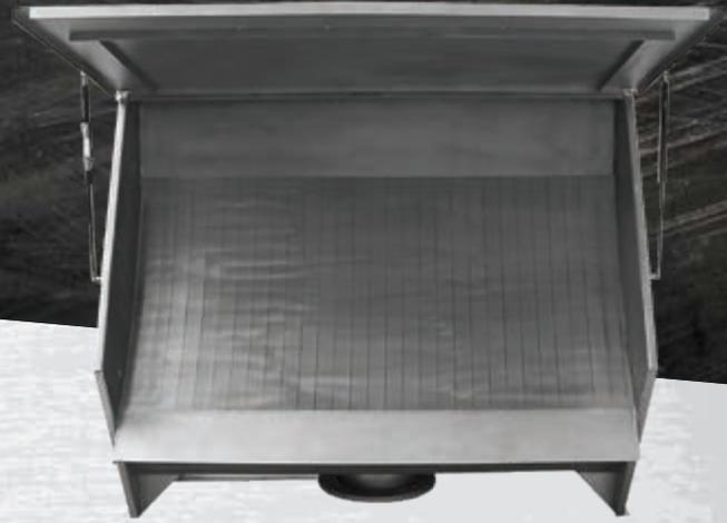
The simplicity of Sidehill Screens make them an excellent choice for static dewatering screen applications. With no motors or moving parts, the Sidehill Screen lets gravity do the work as effluent flows down the screening media.
